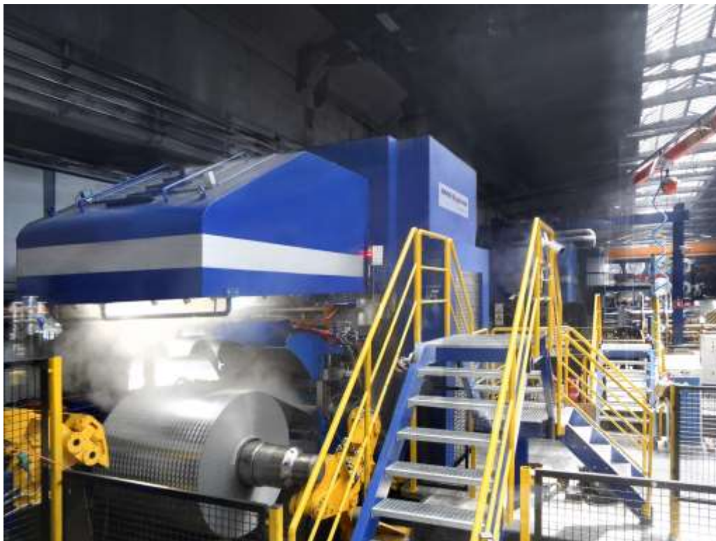
Treadplate production on the aluminum cold rolling mill revamped by SMS group.
