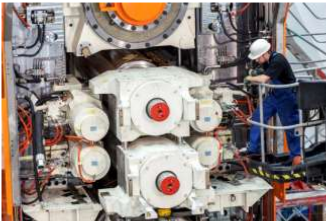
Pre-assembly of a CVC ® plus system in the SMS group workshop.
