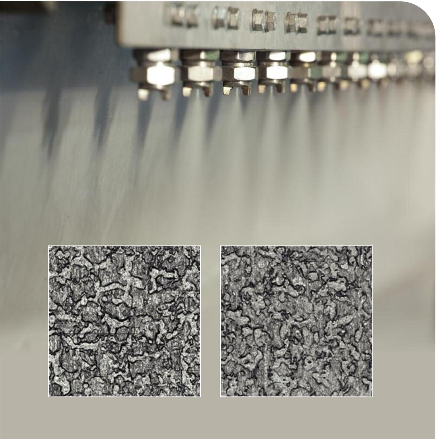
A direct comparison with a dry-skin-passed strip (r) shows that the strip skin-passed with ECOLub features comparable roughness without lubricant impressions on the strip surface.
