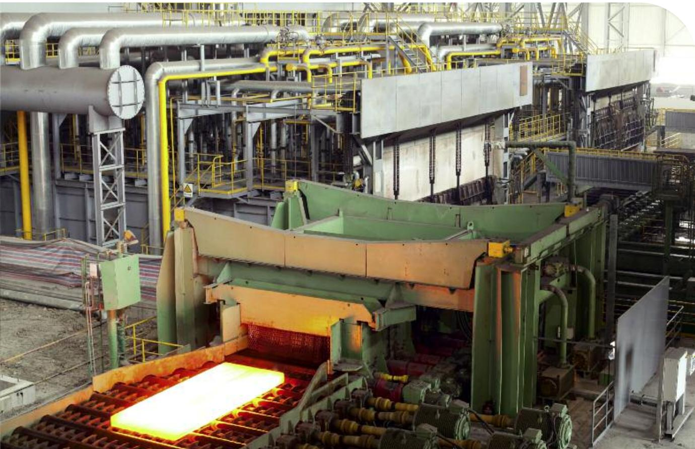
Descaling unit with 1,000 mm roll lift for descaling ingots.
