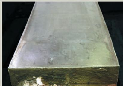
Copper with UniGuard® Coating after 342,000 tons
