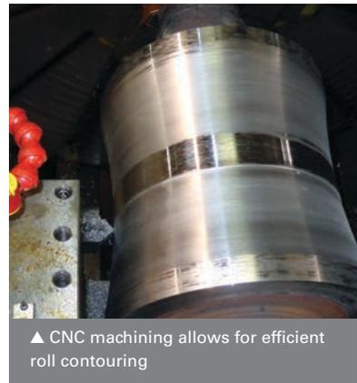
▲ CNC machining allows for efficient roll contouring
