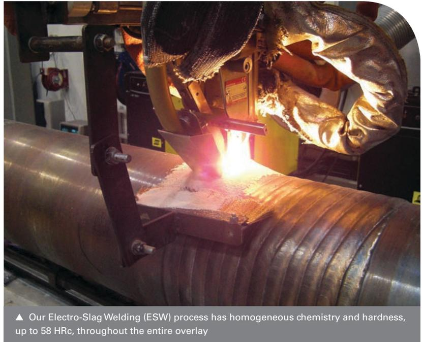
large liquid pool, overlay chemistry and hardness is extremely homogeneous. As a result, rolls that have been clad with our ESW strip process have better wear profiles; longer service lives; roll runs between regrinds are longer; and mill downtime for roll maintenance is less frequent.
