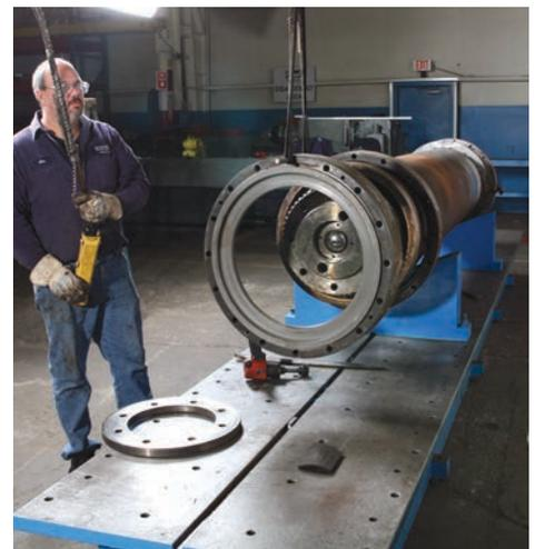
▲ Spindles are carefully disassembled following stringent procedures
