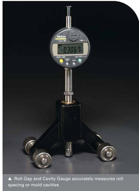
units. A .400-inch tip extension for use in caster molds is also available
