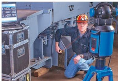
▲ Laser measurement system provides accuracy to 0.0004 inches
