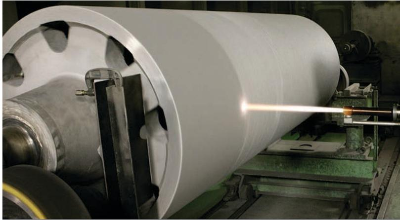
▲ Zinc pot rolls coated with our system have increased resistance to corrosion, wear and zinc dross adhesion
