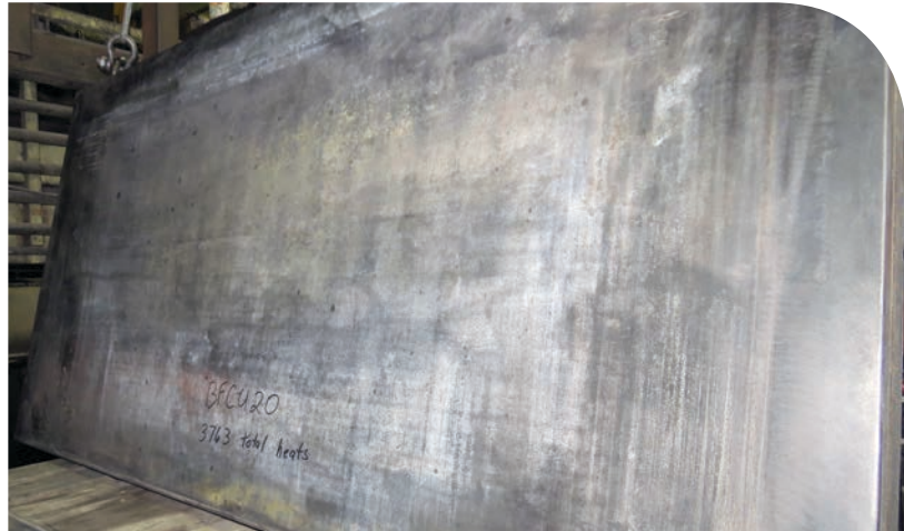
▲ After being in service for more than 500,000 tons, this broad-face copper coated with our UniGuard® Coating was returned to service
