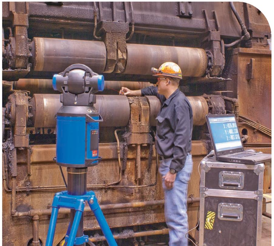
▲ Equipped with a 3-D laser measurement system, our technicians can align, inspect and set-up equipment faster and more precisely than ever before
