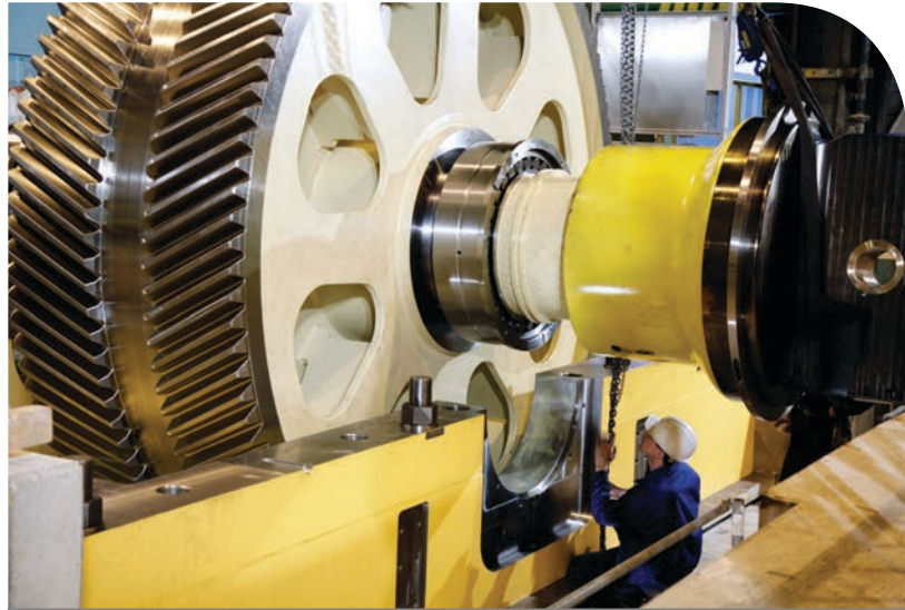
▲ SMS group engineers check and verify the contact pattern and backlash on gears we reassemble to ensure they meet exacting OEM specifications
