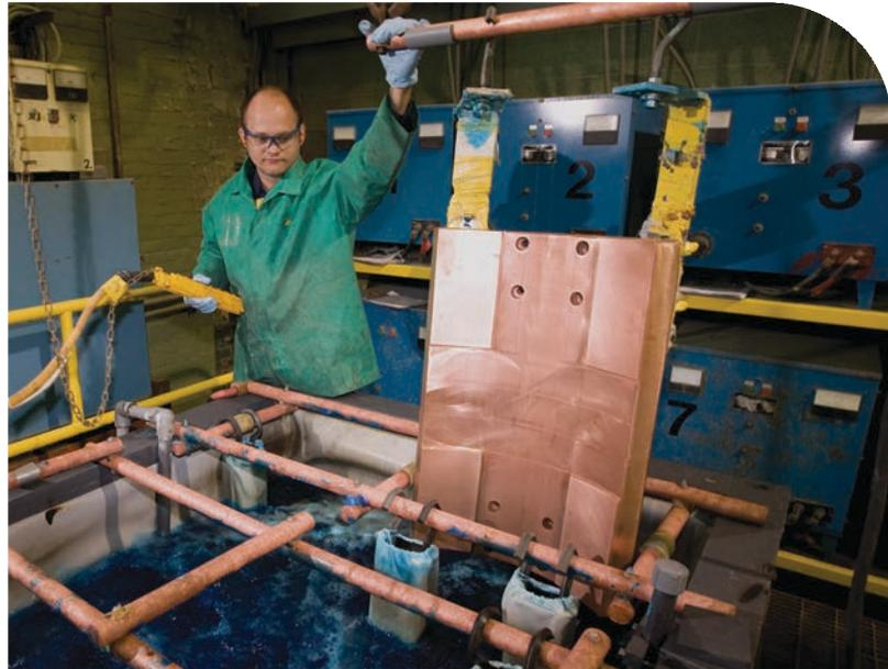
▲ Repairing copper castings using copper plating is far superior to repairs made with copper welding
