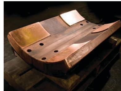
▲ Castings rebuilt using copper plating last as long as the original casting
