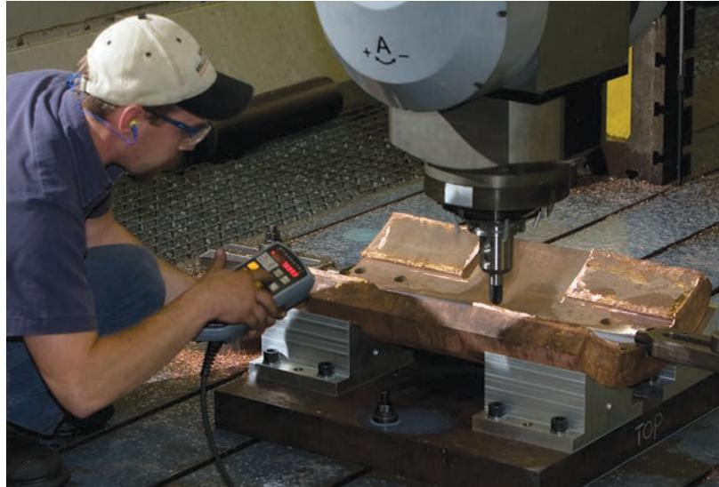
▲ Machinist precisely indicates the pad surfaces on an electrode holder before final machining
