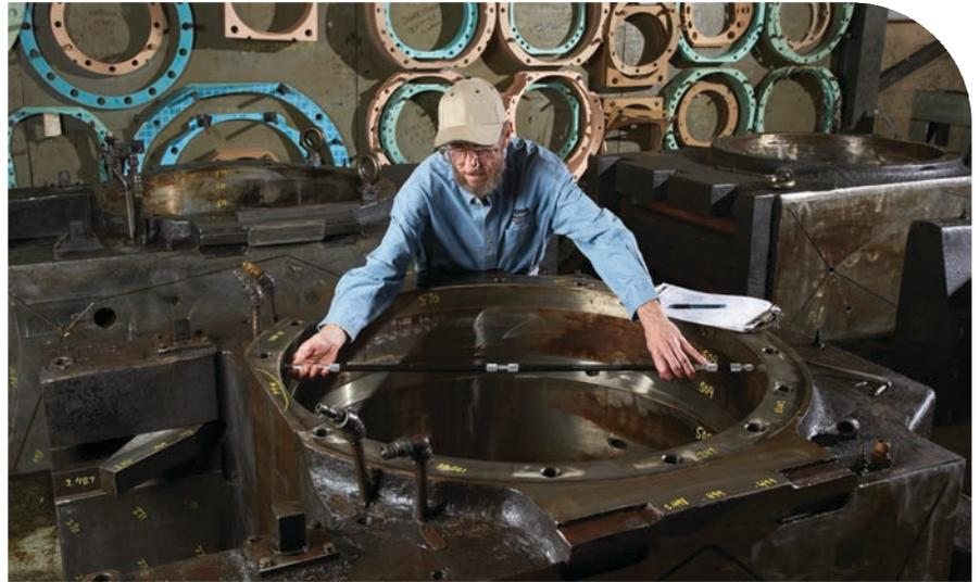
▲ During incoming inspection, chock dimensions are carefully and precisely measured
