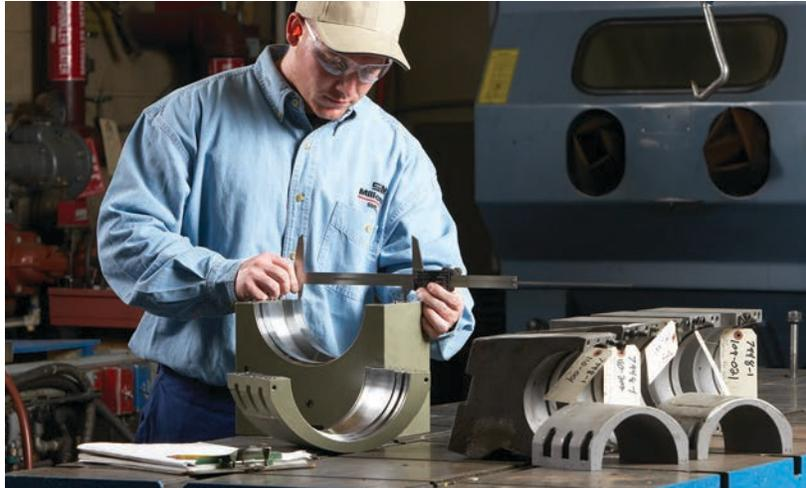
▲ Bearing housings are precisely machined and carefully checked to ensure top performance
