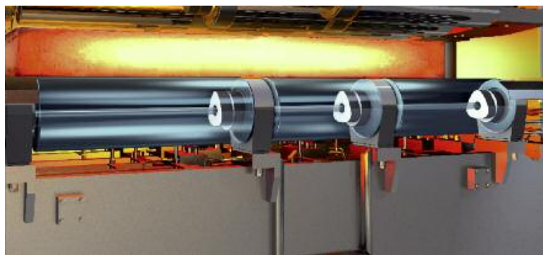
STEC-Roll® with internal cooling via central bore ...
