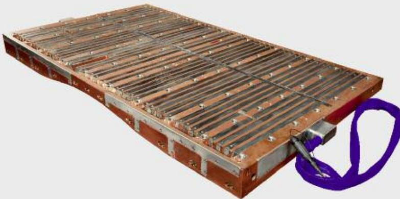
HD mold with integrated sensors.
