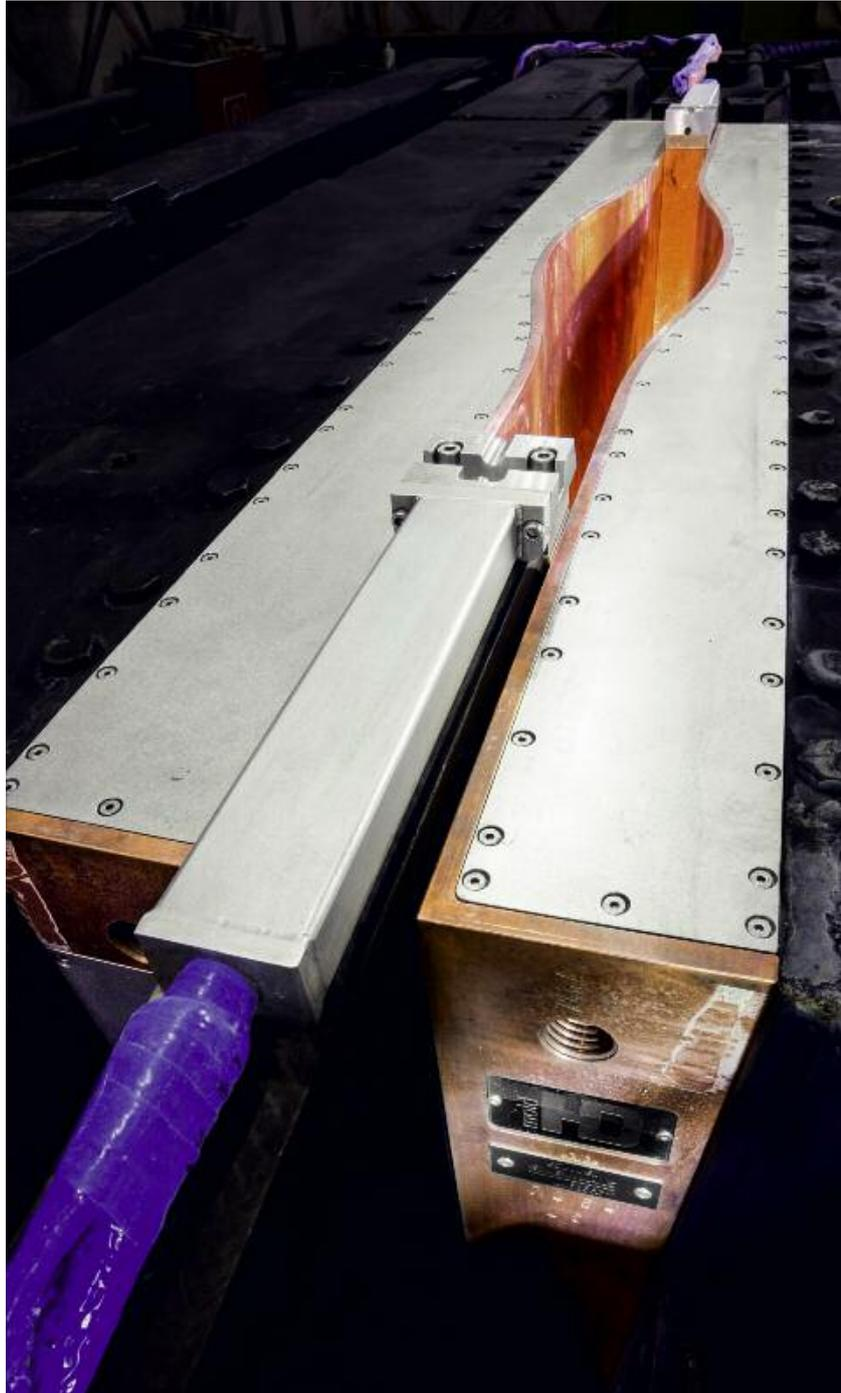
HD mold in a CSP<sup>®</sup> casting machine.
