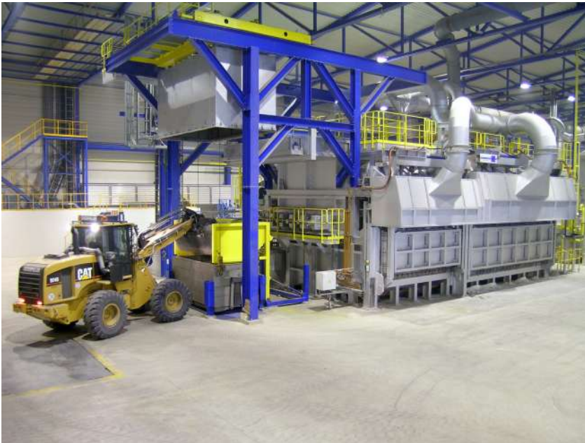
Multi chamber melting furnace Ecomelt-PS.
