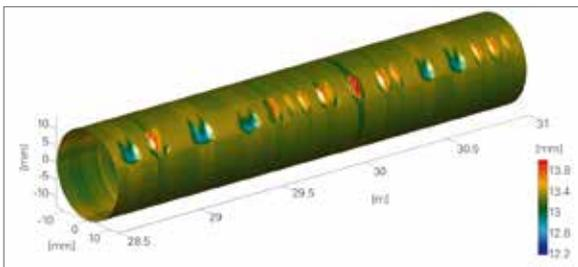
Deviations that occur frequently though irregularly indicate defective ingoing material.
