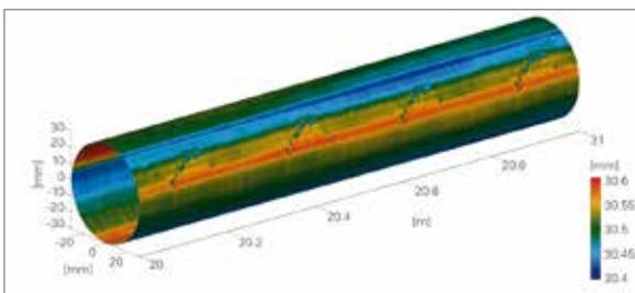
Periodic deviations are caused by damaged rolls or guide rollers
