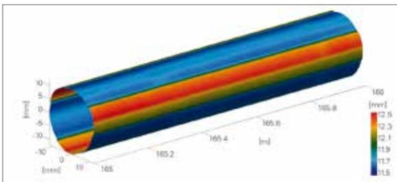
The seams and edges across longer areas of the bar are reduced by adjusting the roll positioning system
