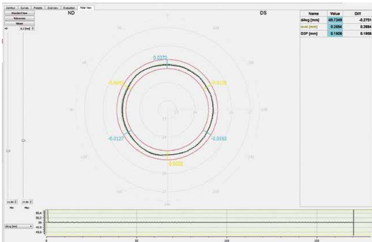
Visualization of rolling results by a MEERgauge® behind the PSM®
