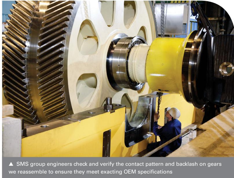
▲ SMS group engineers check and verify the contact pattern and backlash on gears we reassemble to ensure they meet exacting OEM specifications
