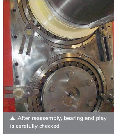
the unit is reinstalled in the mill. We also provide laser-alignment services to ensure precise alignment.
