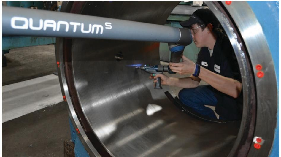
▲ During inspection, chock dimensions are carefully and precisely measured
