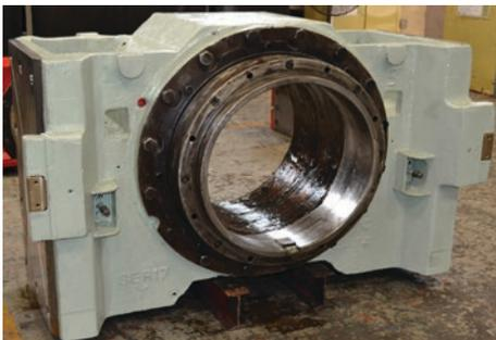
▲ To ensure chocks reliability in the field, they are precisely machined
