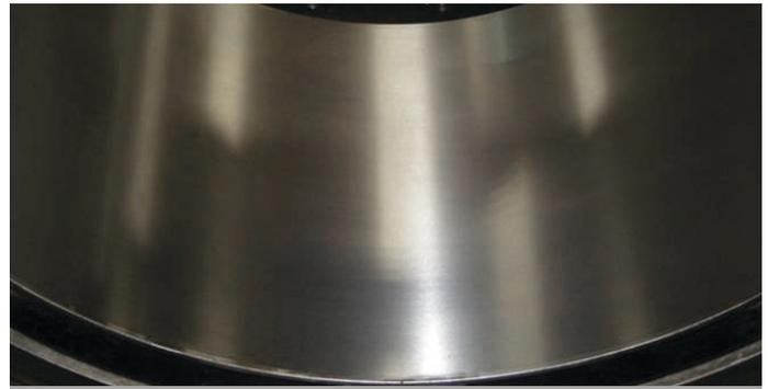
▲ Work roll chock after final machining
