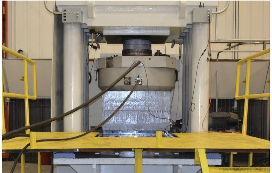
▲ Because the test stand has state-of-the-art computer controls, we can accurately and reliably test large AGC cylinders against their OEM specifications
