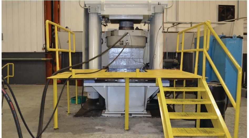
▲ With one of the largest computerized test stands in North America, we can test AGC cylinders from all manufacturers up to 66 inches wide and 57 inches high
