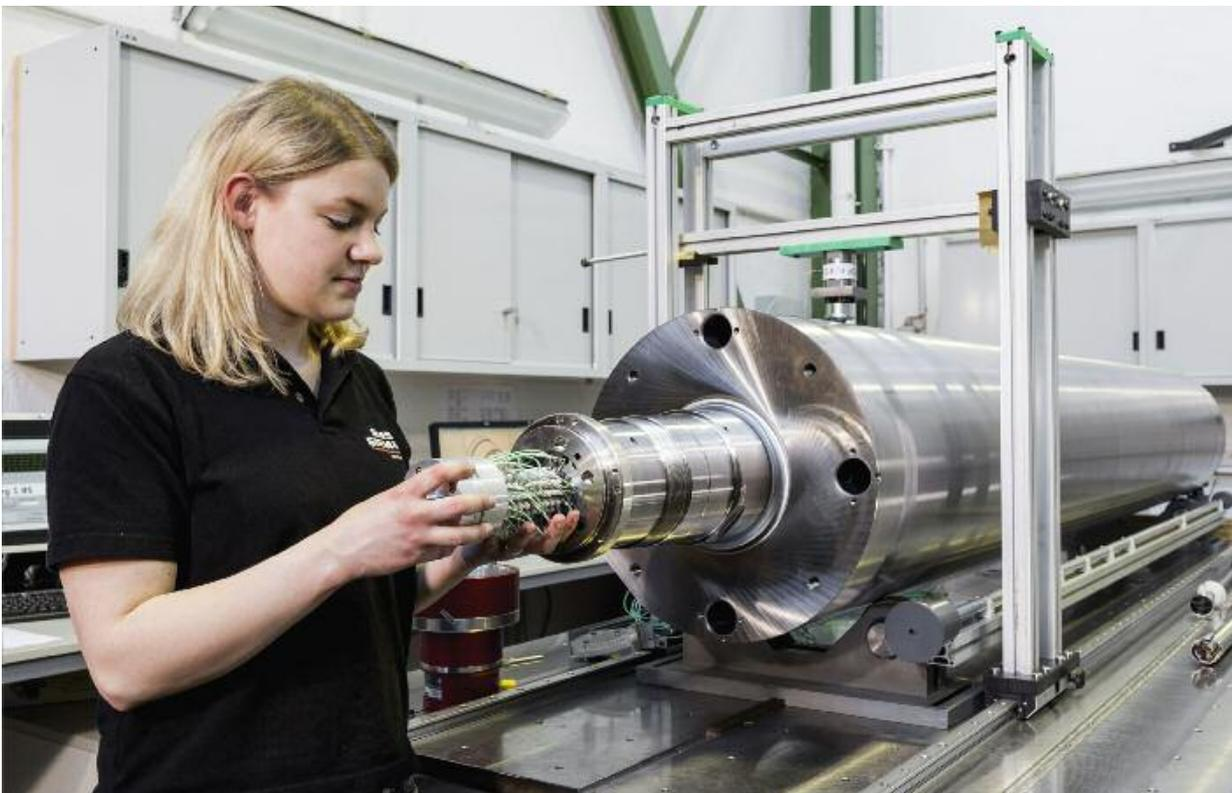
Installation of the signal transmitter.
